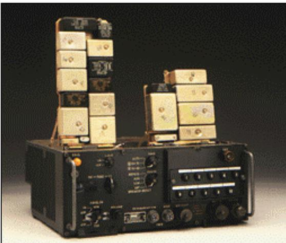
In addition to the conventional noise-operated squelch, an advanced tone-operated squelch (150 Hz) is provided in this series, thus eliminating "false alarms" or undesired audio output from the receiver when net stations are not called. The tone squelch also ensures reliable retransmission when two receiver-transmitter are used as an automatic relay station in high-density communication centers where off-frequency signals often cause false triggering of the retransmission setup.
